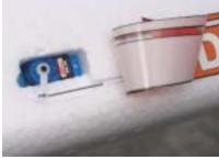
The servos are mounted in molded pockets behind the cabin area. Make sure that the servo operation and control deflections are all correct before you seal the servos into place with the decals.
