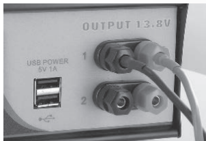
4mm bullet connectors plug directly into most power supplies.
