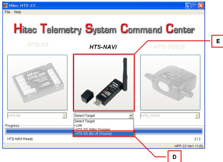
After selecting the proper sensor station, turn on the linked transmitter. Sensors data display window will pop up (as shown by F). Click YES and turn the power on in your Plane or Car where the sensor station is, the sensor data screen will now appear.
