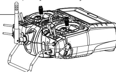
2. The receiver antenna should not be placed near the engine, metal parts or high current batteries.
