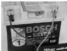
Using a terminal clip attached to a car battery
