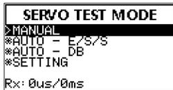
Use the Adjust Dial to select the desired test function. Once the function is highlighted, press the Adjust Dial to enter.
