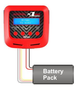
BATT/PROGRAM BATT RESISTANCE Press the START/ENTER button to access the Lithium Battery Resistance program.
